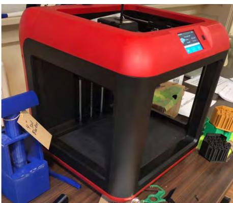
**3D printer**- This printer has the ability to print 3D files in PLA to make customizable farm equipment, replacement parts, and prototypes. It can print objects up to 6" x 6" x 6". This has been used to make seed wheels, seed processing equipment, emt clips for plastic and many other small tools and adaptations for the farm. Please connect with Jacki Perkins at [jperkins@mofga.org](mailto:jperkins@mofga.org) if you would like to have files printed at MOFGA.
