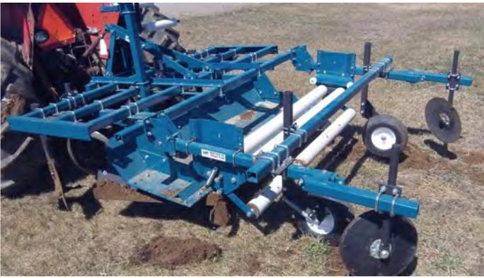
**Buckeye Tractor's 2212 Mulch Layer/Bed Former with drip irrigation** attachment is rugged and versatile. It can prepare beds 2-4 ½' wide and as much as 6" high. It can handle plastic mulch up to 6' wide. It can be used to just form beds without mulch. It uses a category I three-point hitch and requires 45 horsepower. It's about 8' wide and weighs roughly 1200 lbs.
