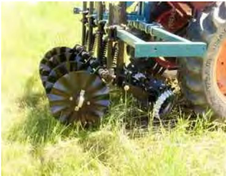
The **Strip Tiller**- was built at MOFGA with two row cleaners and four 13-wave coulters on a 7-foot wide frame. This unit is intended to create a planting strip in one pass and is easily adaptable and adjustable to a variety of situations. On smaller tractors the distance between rows may be fixed, but in larger tractors there is more variability with this unit.
